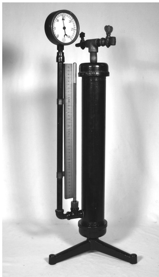
Boyles Law Apparatus. This is listed in a 1921 Cenco bulletin as being designed by a High School Teacher for high school teachers. The glass tube, partly filled with oil, is connected at the bottom to the iron cylinder, also containing oil. The scale beside the tube gives the volume of the air trapped in the glass tube and the dial gauge records the pressure at the bottom of the tube (no correction is made for the head of oil in the tube). The pressure is then modified with a vacuum or pressure pump, and a graph of the pressure as a function of the reciprocal of the volume is a straight line. The apparatus was designed by Walter R. Ahrens of Englewood High School in Chicago and cost $25.00. (Notes and photograph by Thomas B. Greenslade, Jr., Kenyon College.)
